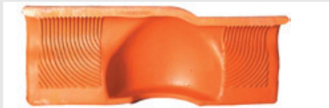
*Sectional view of typical insulator cover showing arrangement of ribs. Ribs are engineered to grip the serrations on its corresponding line hose, regardless of angle.*
